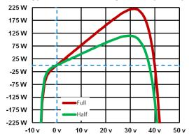
The major feature of this profile is the existence of a single, maximum power point. The point will shift right and left with temperature.
